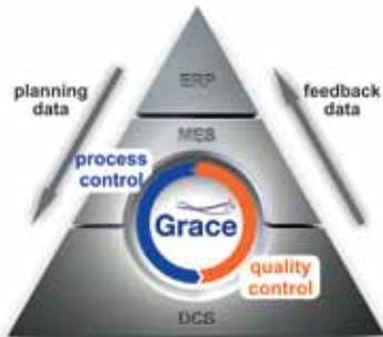
The Grace system will act at the Distributed Control System (DCS) and Manufacturing Execution System (MES) levels, implementing the sharing of process critical information between and inside the two layers. This results in a more efficient management of resources and a higher final product quality.
